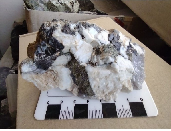
Pegmatite mineralized with fluorite+cassiterite, sulfides, stannite and Bi-minerals, Verněřov
